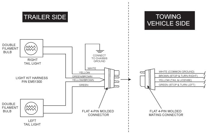
Figure 34. Trailer Tail Lights Wiring Diagram
